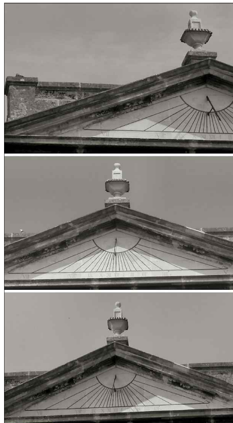
Fig. 2. Top to bottom: photos taken am, noon and pm on 29 th July 2006 to show the track of the sunlit triangle across the face, and to capture the morning moment when the gnomon shadow just begins to show the time and the afternoon moment when it is just about to switch off.
