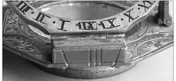
Fig. 1. File marks crossing the hinge and dial plate of an Augsburg dial by Lorenz Grässl.
