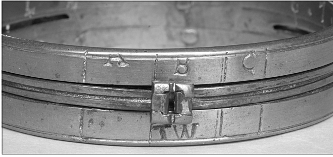
Fig. 3. Poke dial stamped 'TW'. Note the misalignment of the letters 'A', 'B' and 'C' which is identical on all known dials by 'TW'
